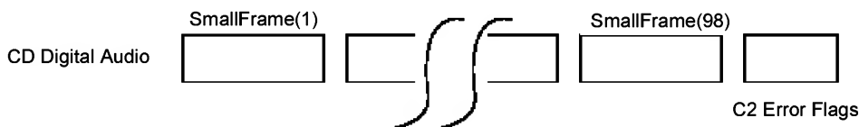
Fig. 1.22. Sequence of frames making up a block
